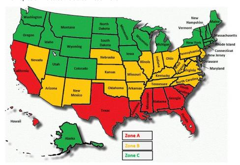
Zone A - States with high temperature cycling and humidity (includes Puerto Rico, Guam, and Saipan). Time in service until significant propellant degradation may occur is projected at between 6-9 years.
