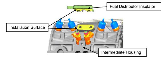
2. Also, prior to installing the fuel distributor on the fuel distributor insulator, be sure to clean the installation surfaces prior to tightening the bolts.
