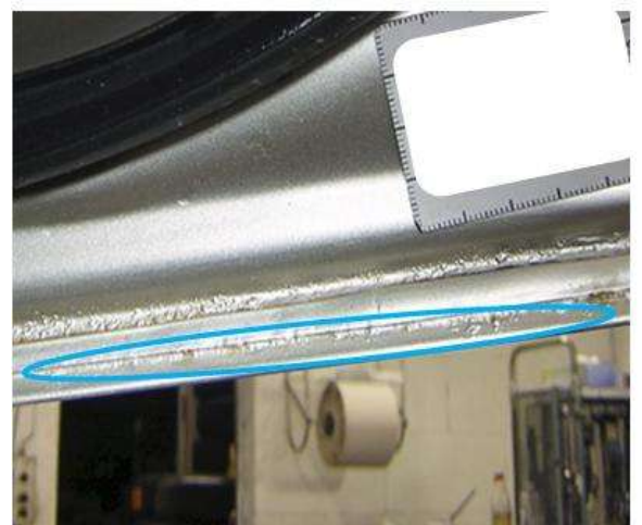
Visible blisters appearing between outer edge of sealer and lower outer edge of door.
