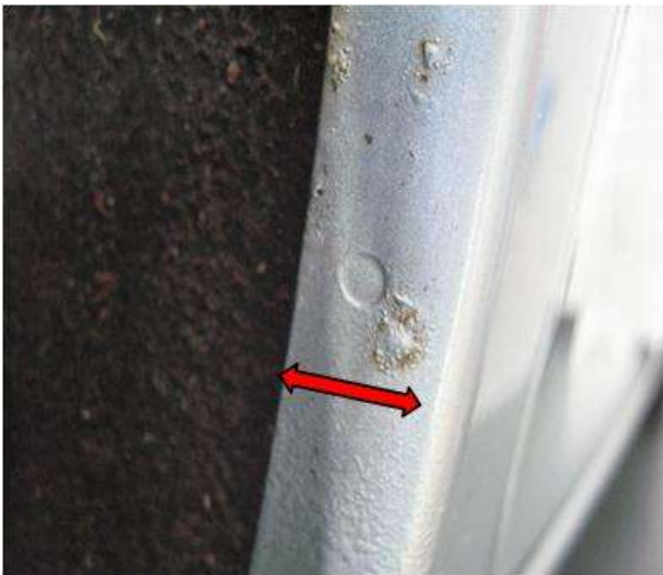
Single blister caused by chipping in an area more than 10mm from the inner edge of the wheel arch arch.
