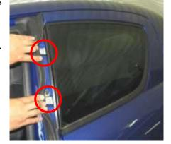
2. Open the rear door and pull the door glass lever to open the door glass.
