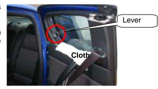
3. Attach a piece of non-woven fabric (10 mm x 30 mm) to the upper front of the door glass. (See the following picture.)
