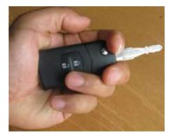
5. Pull the key to confirm that the key does not come off from the transmitter. If it still comes off, then replace the key with a new one.
