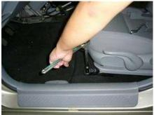
Service Points When Tightening Seat Slider Bolts:
