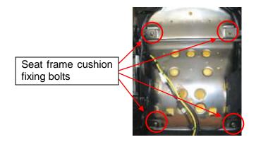
3. Detach the edge of seat cushion trim from the seat cushion frame groove to remove the seat cushion frame. Then replace the seat cushion frame with a new one.
