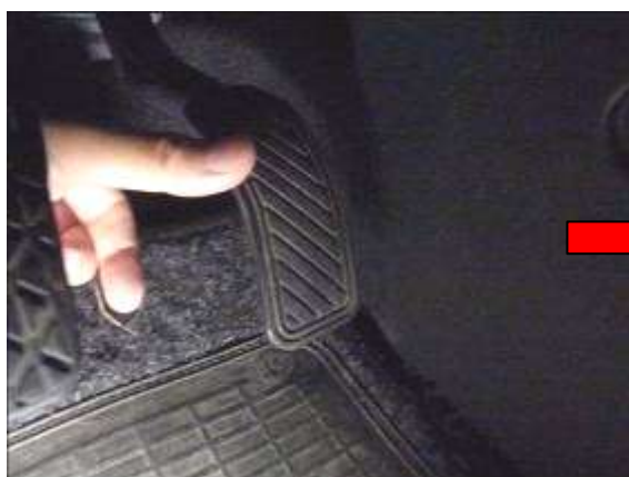
Pedal interferes/overlaps with the edge of the heel pad.
