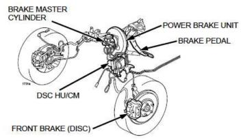
If you encounter a customer complaint for this concern, explain that the noise comes from the ABS/TCS/DSC "Malfunction Detection Function" initial check. The initial check is a necessary function to ensure the normal operation of the ABS/TCS/DSC.
