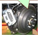
As necessary, polish the disc plate like this. (Wrap the box-shaped wood with sandpaper and rotate the disc to polish.)
