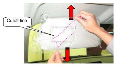
3. Tear the protector and break the welding line on the end so that the protector can be laterally removed on next step.
