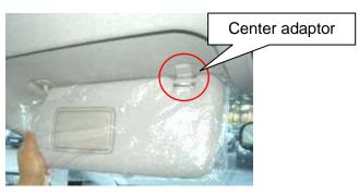
2. In order to avoid any unusual force gets transferred to the stay, pinch the protector and tear it vertically from the cutoff line on the center of protector.
