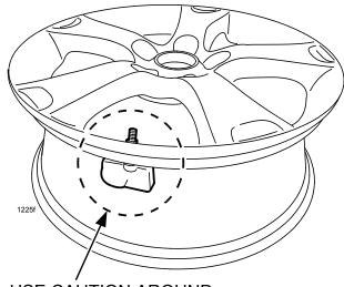
USE CAUTION AROUND SENSOR AREA WHEN INSTALLING TIRE
