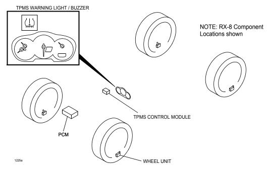
The wheel units are sensors, which are part of the valve stem and are mounted to each wheel. Each wheel unit consists of an internal battery (designed to last up to 10 years), an accelerometer which turns the wheel unit on over 25 km/h (16 mph), a temperature sensor, a pressure sensor and a radio transmitter that sends information to the TPMS control module.
