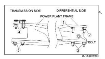
Tighten nut 1 until the power plant frame is seated in the rear differential.
