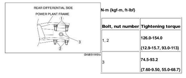
8. Tighten the nuts on the rear differential side in the order shown in the figure.
