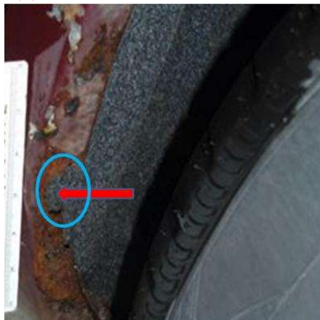
Visible blisters and red rust in an area more than 10mm from the inner edge of the wheel arch.
