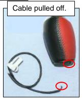
In case of not following above mentioned description the harness will be pulled off and can't be repaired anymore.
