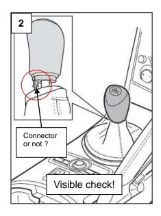
Open button from leather boot and check cable connection. If connected by connector just disconnect and continue with step 3. In case the cable goes directly to the inside of shift knob without separate connector than follow step 4 to 7.
