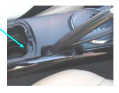
3. Insert a plastic spatula (or equivalent tool) under the removed location. Release the locks and remove the whole shift panel.
