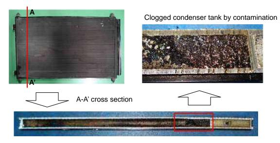
In order to avoid serious damage and costly repair of A/C system, always make sure to use designated refrigerant and compressor oil when necessary to replace or refill.
