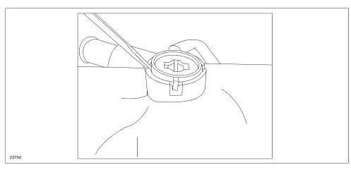
**NOTE:** If the sensor is hard to remove, cut the dotted line (A) as shown (both sides) using cutting pliers, then remove the sensor from the coolant reserve tank using a flat screwdriver (B).
