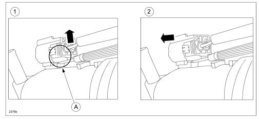
c. Use a flat screwdriver to pry the sensor loose (on both sides) from the coolant reservoir; the sensor will be reused.
