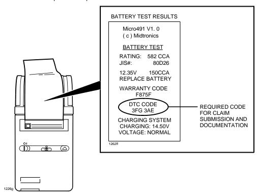
9. Write the 6 character DTC code on the RO and attach the printed results to the RO Hardcopy (do not attach with tape due to reaction with the printer paper).
