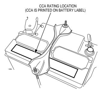
4. Enter the correct battery rating by using the UP and DOWN arrows to scroll to the correct rating, then press ENTER to start the battery test.
