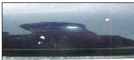
Mark of coating removal caused by flying stone. (Hood)
