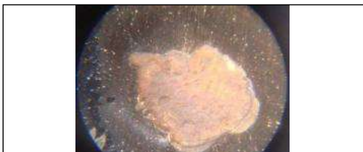
Right after the peeling, impact area is burned and whitened. Edge of peeled area is scraped off at a sharp angle.
