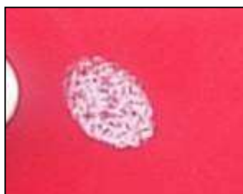
Due to high temperature under the sun, acid in the waterdrop was condensed and penetrated into the paint coating, causing the depression.
