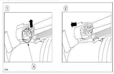
Use a flat screwdriver to pry the sensor loose (on both sides) from the coolant reservoir; the sensor will be reused.
