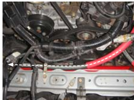
... then route the oil line through the engine compartment as shown and connect to the INBOARD fitting on the passenger side cooler.
