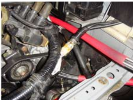
Attach the 45° connector to the adaptor on the rear of the engine. Route the oil line under the wiring harness...
