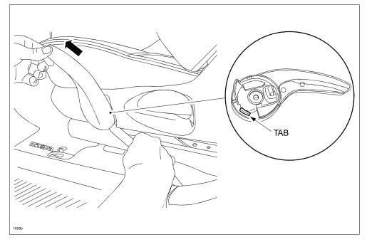
3. Remove the recline lever cover by lifting the lever up and pulling, then remove the side cover screw.
