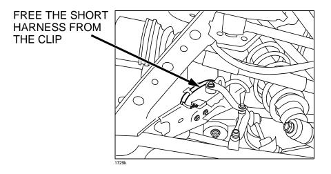
4. Install the new short harness. Ensure the clip is securely installed.
