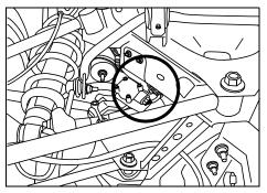
2. Apply waterproof urethane sealer (locally sourced) between the harness and the connector as shown to prevent water instrusion.
