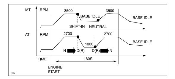
Before turning the engine off, allow the idle to stabilize after the 180 second fast idle duration. This will ensure the engine will start during the next cold engine start-up.
