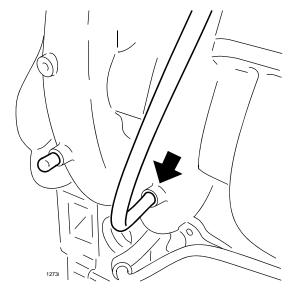
3. Disconnect vehicle barometric pressure sensor connector.
