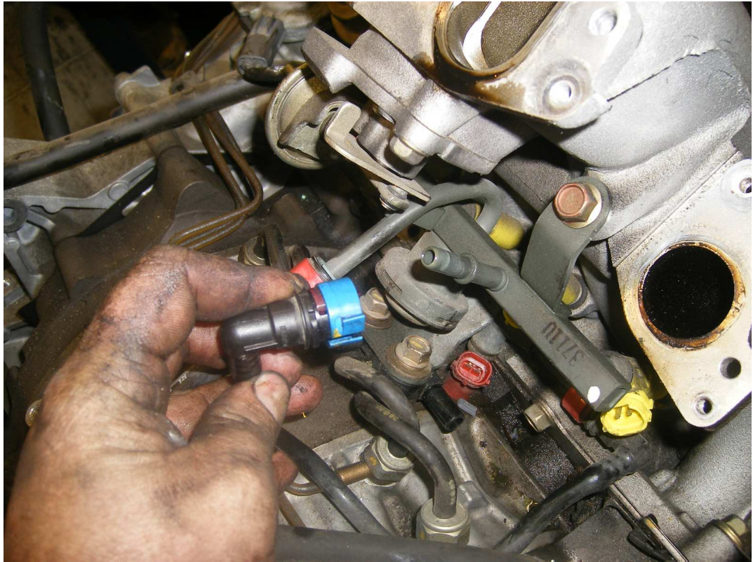
Unbolt and remove lower intake manifold, being careful of auxiliary port sleeves that come out of the block with the manifold. Sometimes it takes several tugs and pushes to get these out of the block when they are stuck due to carbon. On rare occasion I find a stuck sleeve that will not come out of the block, and in this case generous amounts of penetrating oil (wd40 etc.) sprayed down the appropriate intake runner and between the block and gasket/manifold, as well as gentle prying and rocking of the manifold will eventually help get it out.
