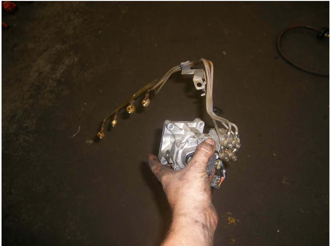
remove the mostat housing and lines as a unit.
