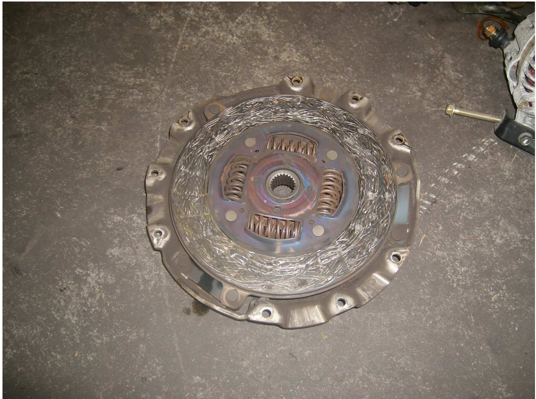
Remove clutch and flywheel. If you are sending an engine to me (or most other engine builders) you can leave the flywheel in place for me to remove for you, as it requires a special socket to remove, so it is understandable if individuals cannot remove it themselves.
