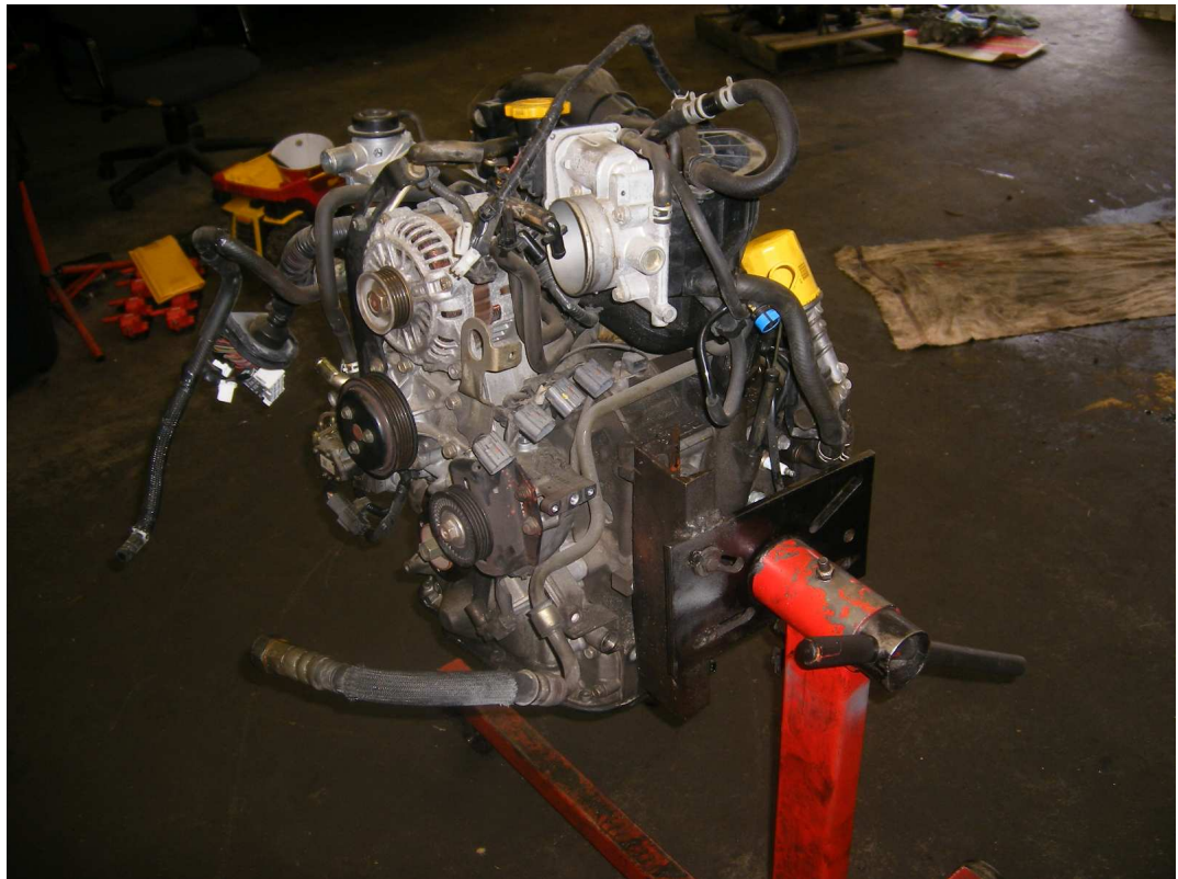
Unbolt knock sensor from rear rotor housing. Remove spark plugs. Use a 24mm socket to remove the oil pressure sending unit.
