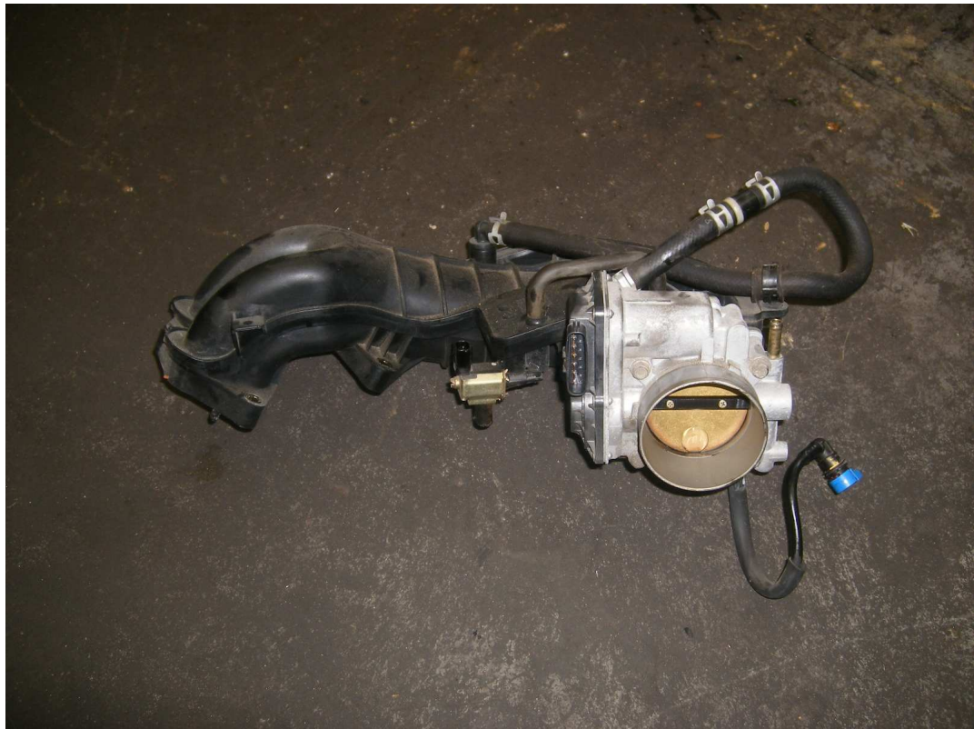
remove oil filler neck. Remove 3 solenoid plugs from the back, 2 vacuum solenoids from port actuabrs, harness clip, and 2 nuts at base of the neck.
