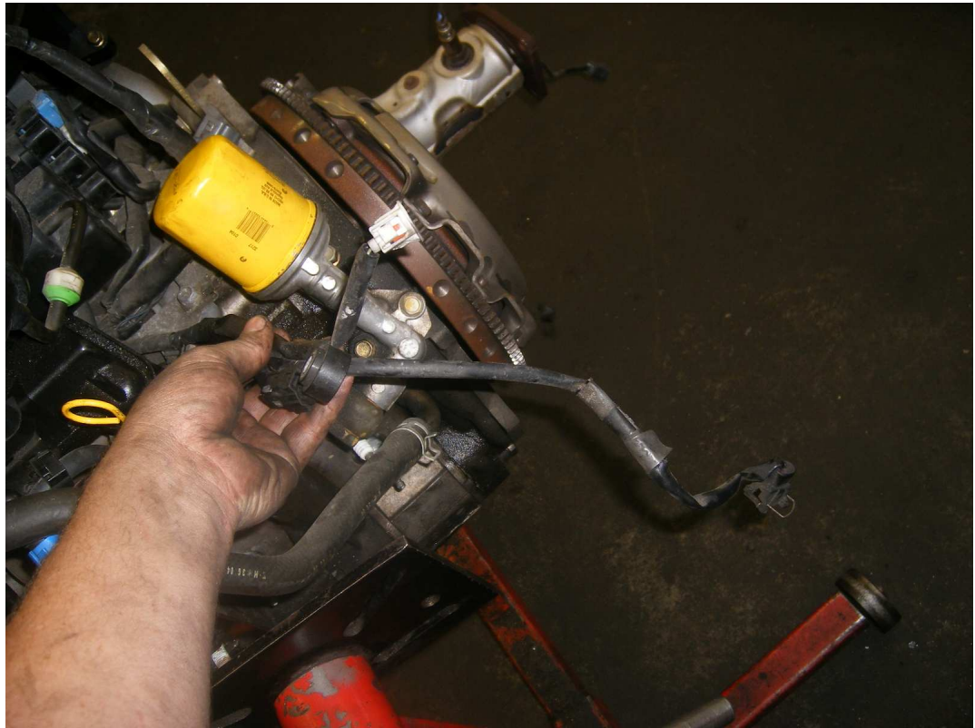
Remove rear heater core hose from pipe on rear iron.
