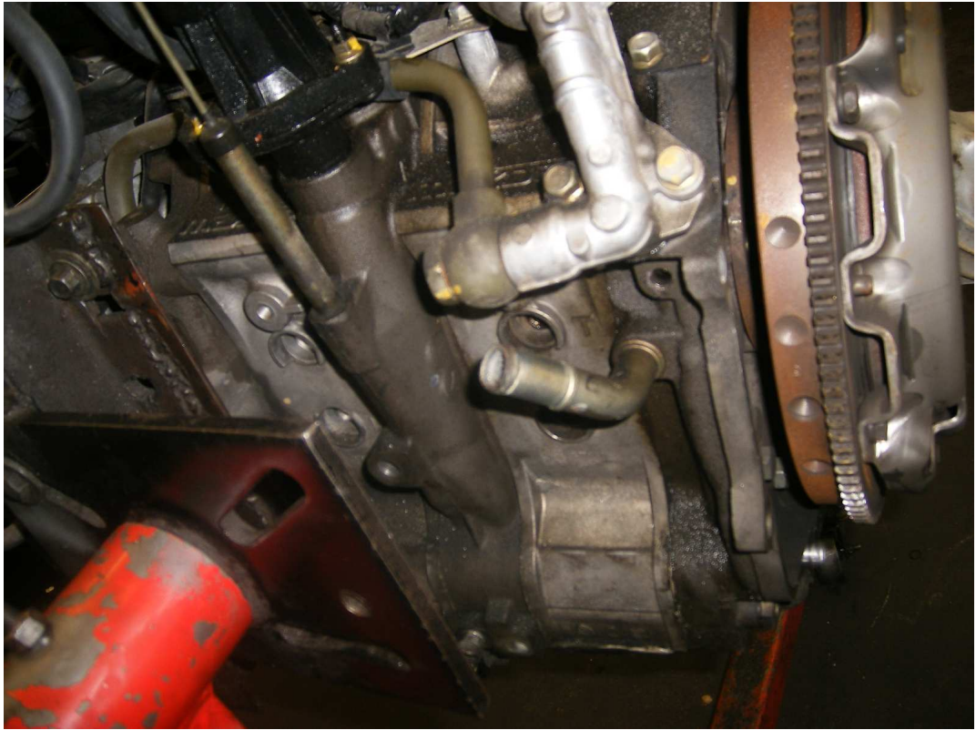
Remove air control valve...disconnect vacuum hose, remove bolt on top bracket and 2 nuts/studs on exhaust manifold. Disconnect wiring harness clip. On some cars the two nuts/studs on the exhaust manifold will be rusty, or you may want to und off the nuts...in this case it is fine to leave the ACV bolted onto the manifold and remove them as a pair.
