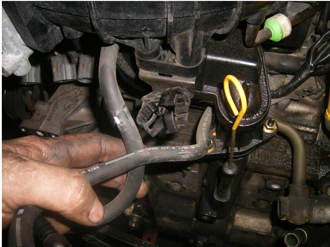
Use a long extension and socket to remove the 2 10mm bolts facing down from the retaining clip under the intake manifold.
