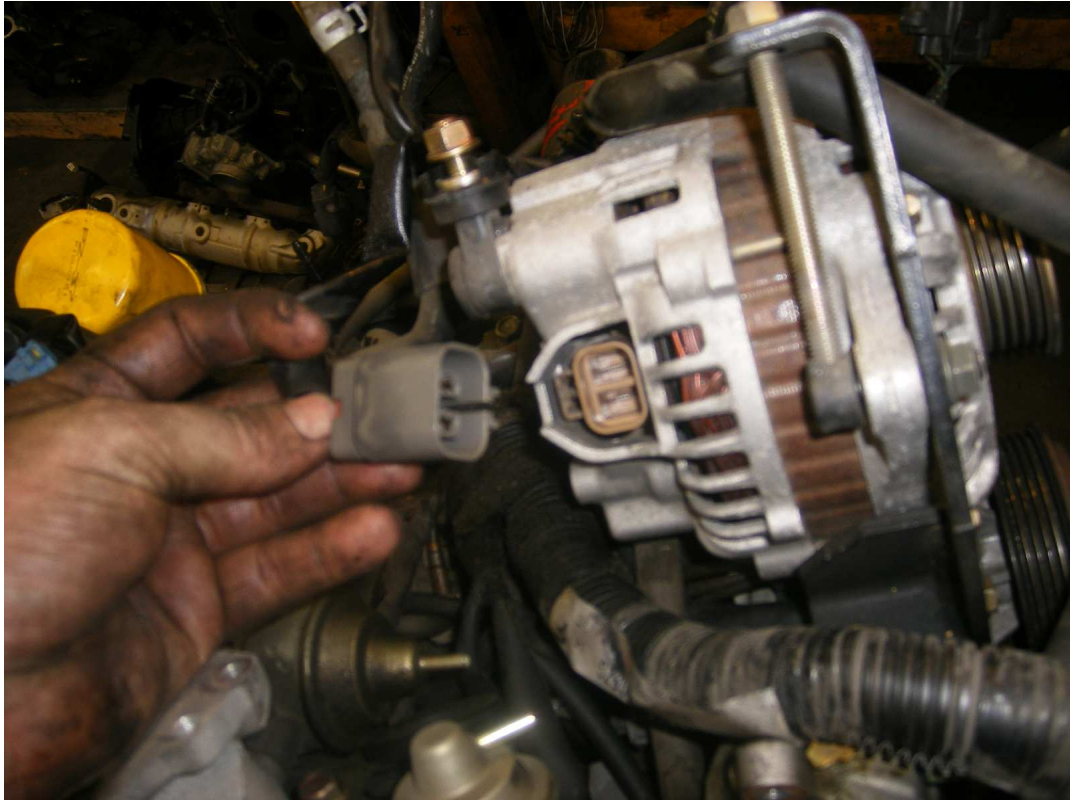
Unplug alternator plug.
