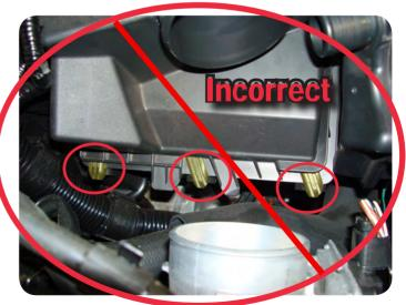
Left side of the air cleaner cover is <u>not</u> inserted into the lower air cleaner housing correctly.
