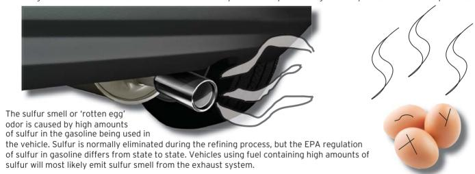
When high sulfur fuel is burned, there is a chemical reaction in the catalytic converter causing the sulfur to oxidize. As the vehicle is driven, the oxidizing reaction odor in the converter will decrease with mileage and age.
