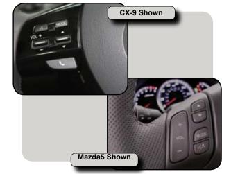
Voice commands may not be recognized depending on the voice. If the voice commands are not recognized correctly, repeat in a louder voice, close window(s) / moonroof, change AC airflow speed/direction, wait for interference to pass.
