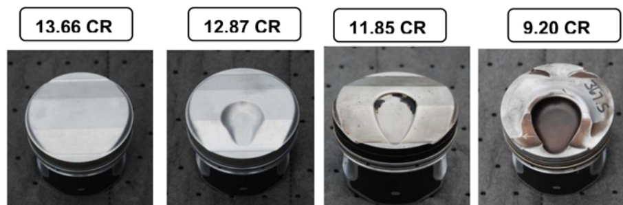
Figure 5. Series of pistons and resultant compression ratios investigated.
