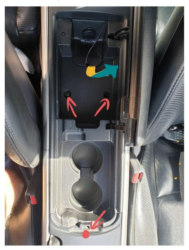
5. Open the DVD/navigation system cover, lift up the fabric, and unscrew the 2 screws. Remove back mid-seat storage place by opening it and lifting it up, to find 2 more screws
