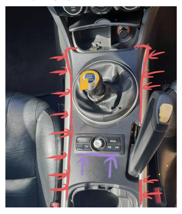
4. Open the middle storage, lift up the fabric, and unscrew the 2 screws. Remove 12V socket by pulling up the bottom part of it, and sliding it out, and finally undo the power connector. Previous step will uncover another screw in the center, remove it as well.
