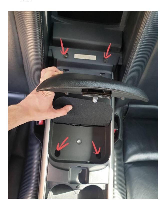
6. Now that all of the screws were removed, the complete central console can be lifted up. Keep in mind it still has plastic clips along the edge. Start by lifting up from the most rear side of the vehicle, going forward, until the complete middle section is separated from the car. Take it outside. You should now observe the following:
