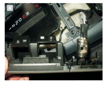
4. Remove the front coin storage tray and power adapter.
