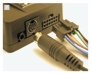
7. Connect the vehicle specific cable's 8-pin molex connector and iPod Docking Cable to the DICE module.
