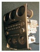
6. Locate the CD Changer wiring harness; this will be on the back of the radio. The DICE vehicle Interface Cable will need to connect to this port.
