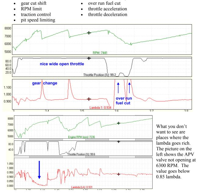
There are 2 different lambda sensors available for your car. One can be read by the MoTeC ADL, the other is read by the MoTeC ECU. Both can be logged in the dash, but each sensor has its own advantages and disadvantages. Either sensor will require the *"lambda option"* in a MoTeC device.
