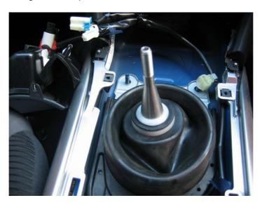
13) The rest is just a reversal of the disassembly. Secure the upper boot, refit the harness clips, connect up your illuminated shift knob (if you had one!) and replace the ashtray. Reconnect your seat warmer/ Audiopilot connectors, replace the covers and knob.....you're done.
