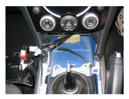
8) With the four 10mm nuts removed, the upper rubber shift boot can now be removed. Gently twist and pry off by hand. Now you can see the lower shift boot, it is held on by love....remove by hand.
