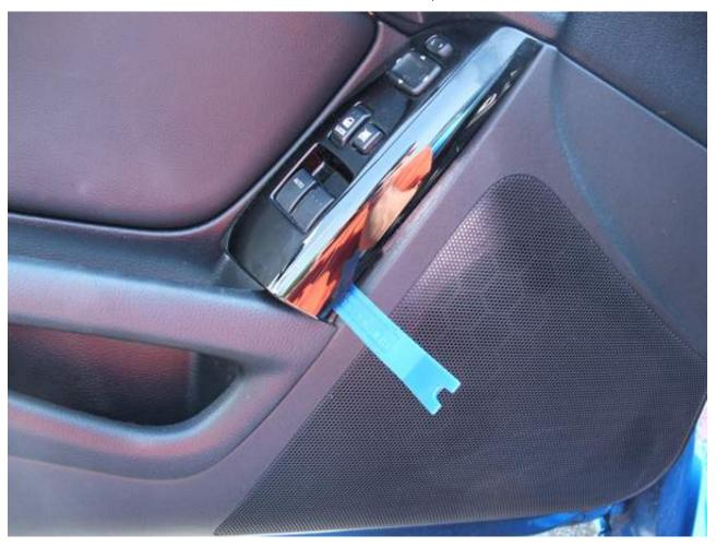
and disconnect the 2 connectors from the panel. Lay this aside so it wont be damaged, we don't want to scratch up the interior panels of our 8 do we?
