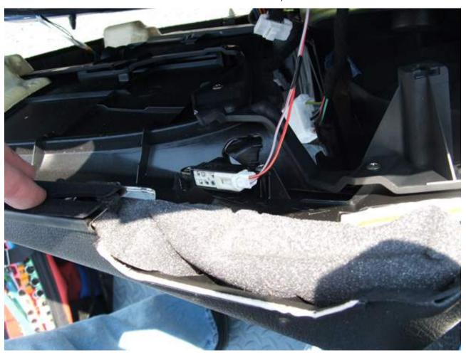
and the light at the rear lower portion of the door. The light pops out by applying slight pressure perpendicular to the direction to which the light is inserted into the door panel.
