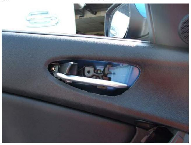
Remove the door panel by inserting your panel popper between the panel and the metal part of the door, gently prying out, while pulling gently as well on the panel, working from the bottom of the door. Once you have popped the panel loose, lift from the back of the panel, keeping it relatively parallel to the door. The door panel should come off relatively easily, but be careful as there are 2 sets of wires connected to the panel still, the LED illumination for the switches
