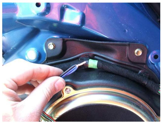
and crimp an insulated spade connector onto the bare wire
