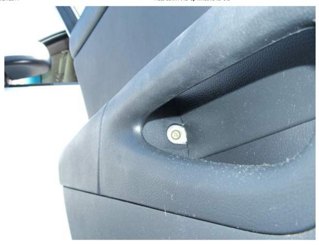
Now remove the bezel around the interior door handle by sliding forward slightly and then prying up gently from the front, and work around door handle and lock
