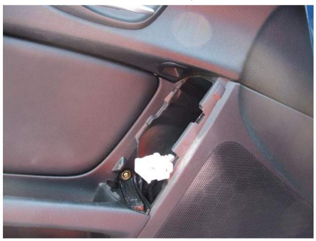
Now remove the screw behind the interior door handle by first gently prying up the little circle cover, then unscrewing screw.
