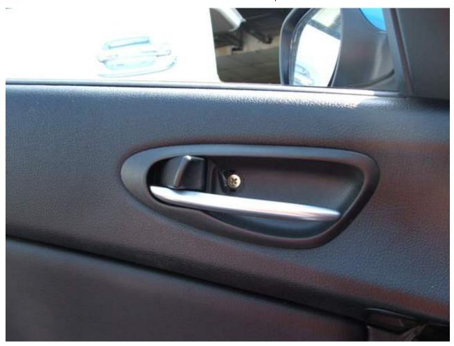
Then remove gold colored screw located behind the switch panel that we already removed.
