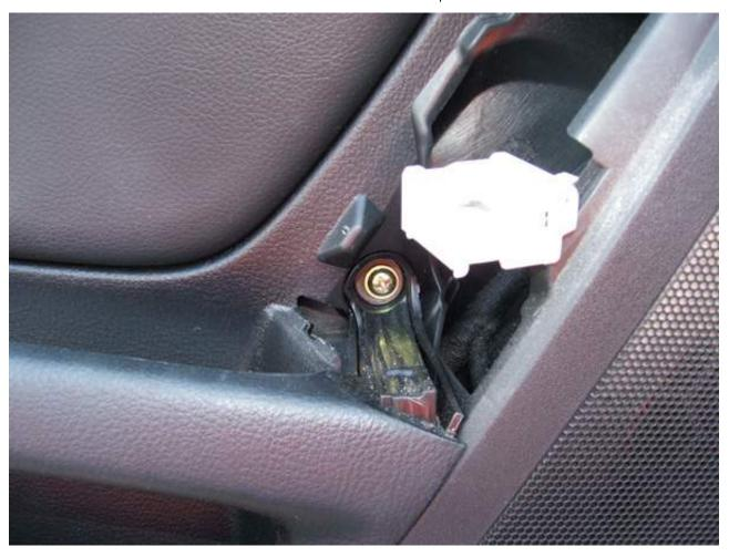
And the last screw we need to remove is the one located underneath the door handle and towards the rear of the door panel.
