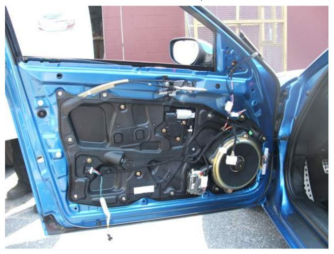
This is where I chose to mount the DEI 530t module using velcro, but for it to fit correctly, you must remove the piece of Styrofoam from the inside of the door panel.
