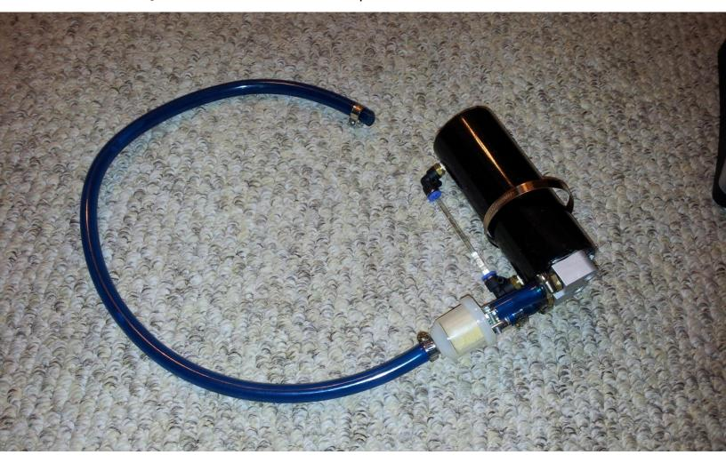
h. Before installation (but after building the bracket below) add some oil to the reservoir and let sit overnight in a warm place, then check carefully for leaks and repair as needed.
