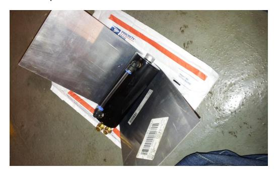
b. Bend the aluminium sheet to make a "b" shape as below. The top of the "b" will eventually mount to the windshield washer tank.
