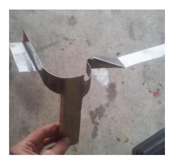
f. This is a bit optional, but add insulating foam to absorb vibrations and keep the metal from rubbing on adjacent parts.
