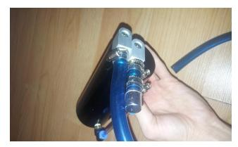
e. Attach the remaining length of hose to the other, unblocked connector.
