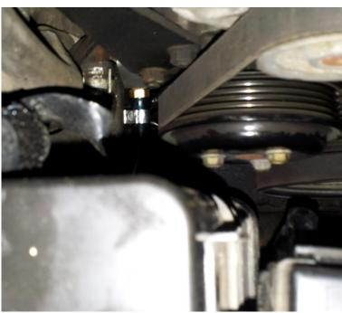
b. Tighten everything down, fill with oil and check for leaks. Be sure to fill the fuel filter completely, to avoid air bubbles. In the picture above, it's not full.
