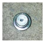
This will feed air into the can as the oil drains. Not having this hole will lead to vacuum in the reservoir, and the OMP will not be able to get any oil from it. Do this away from the rest of the kit to avoid metal particles in the finished product.
