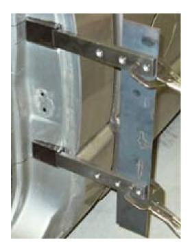
Remove the hinge arms and pull the the hinge pockets out of the holes. You now need to strip the paint from the openings prior to welding. Jason recommends using airplane strength paint remover. Just be careful not to get it on any other part of your car! Mask off all surrounding areas before using the paint remover. Otherwise you may end up ruining your paint job.
