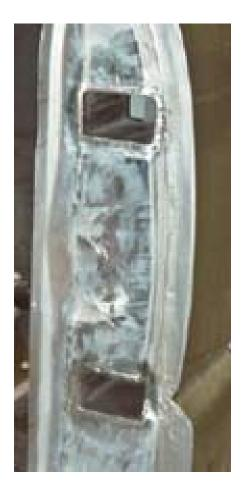
Before priming the surface, roughen it up with some course sandpaper or a sanding disk. This will allow the primer to bond to the metal better. You can use your favorite auto body primer to prime the surface. Jason used a Dura-Build primer. If you are not sure what to use, ask someone at the body shop supply warehouse. They'll gladly assist you.
