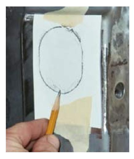
To hold the small circular piece of sheet metal in the hole while you weld it in place, tack weld a piece of metal to the middle of it. You can then hold it by this piece while you weld. After you're finished welding, simply break the piece off.
