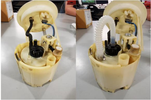
9 – Re-attach the top hat to the bucket assembly and secure with the OEM clips.
