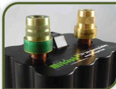
Top Post Adapters Installed
