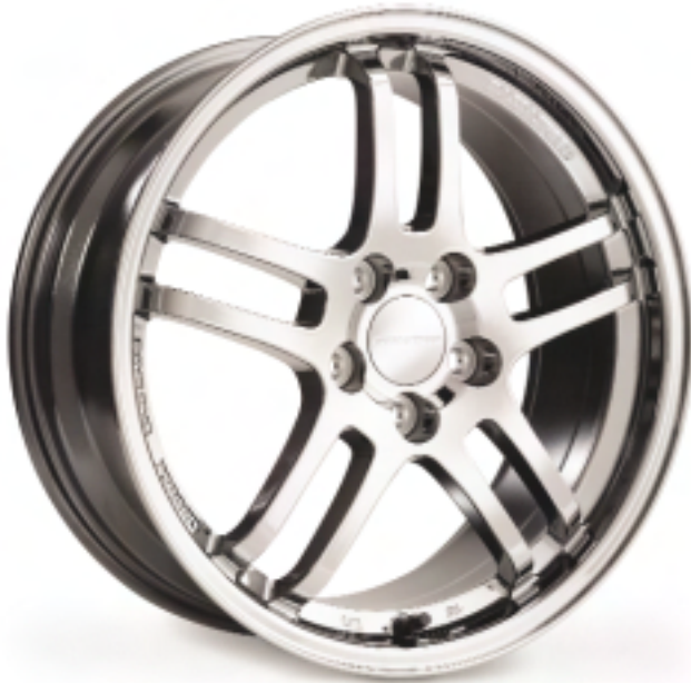
● Forged Aluminum Wheel A MAZDASPEED Forged Light Weight Aluminum Wheel. Reduce the unsprung weight of your vehicle by utilizing these 7.7kg one piece forged aluminum wheels. Reducing unsprung weight improves handling response, braking and acceleration. 18X7.5J Forged Aluminum Wheel (Hi-Light Silver) BLMS-8M-Z01 Forged Aluminum Wheel (Smokey Chrome PVD) BLMS-8M-Z06
