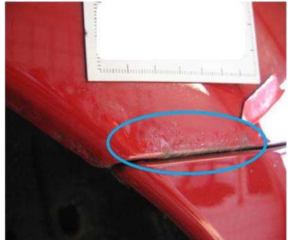
Visible blisters and red rust at vertical surfaces of wheel arch or rear bumper attachment area will not lead to level-3 as long as no proof for perforation can be detected.
