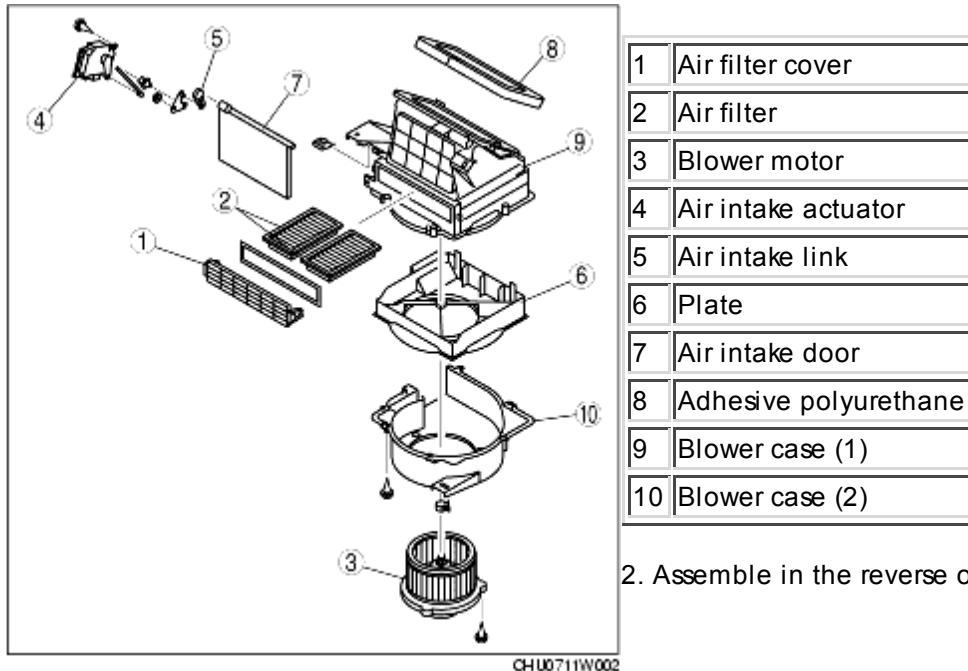
2. Assemble in the reverse order of disassembly.
