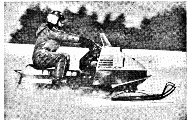
Fig. 5.16 Snowmobile (Outboard Marine, USA, 530cc × 1-rotor)
