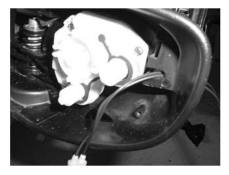
26. Next, place the puddle lamp assembly into the mirror as shown. Note the tab in the recess to the left and the way the mounting hole matches up on the right.
