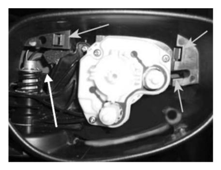
6. Once the clips are released the cover pops off easily. CAUTION: The cover pops off rather easily if all the clips are released ... if it is not popping off easily, double check that you have released all the clips
