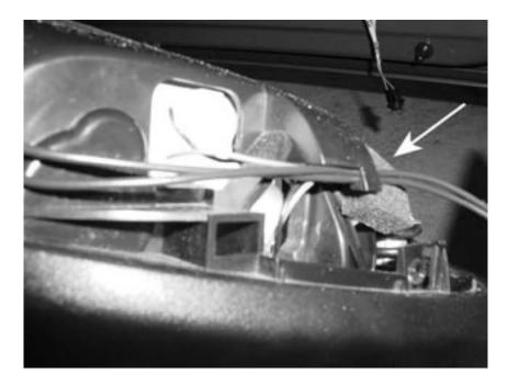
29. Remove the panel show below underneath the mirror to get access to the cable run. CAUTION: This cover pops off with a small screwdriver. The cover is held on by several small tabs that can break if you do not use caution.
