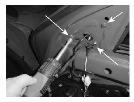
24. With the mirror assembly now free and in your hands, it is time to install the puddle lamp. Shown here are three points of interest inside the mirror. The tab on the puddle lamp assembly slides into the recess indicated by arrow 1. Arrow 2 marks the location where the puddle lamp assembly is screwed to the mirror housing. Arrow 3 shows the slot through which the bulb and wire assembly pass to plug into the puddle lamp housing.
