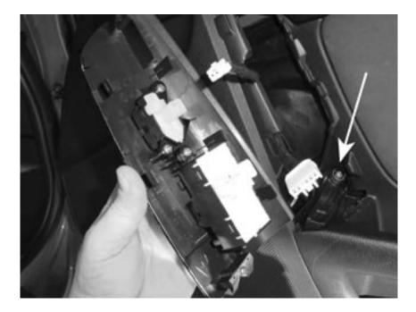
15. The third screw that needs to be removed is at the back of the inner door handle well near the armrest. Use a medium screwdriver to get this last screw out.
