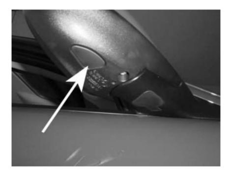
2. Start by pushing/rotating the mirror assembly back towards the front of the car to make it easier to get at the inside.
