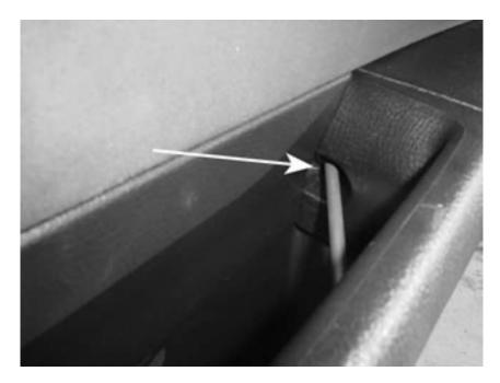
16. With all three screws now recoved, you are ready to pull the inner door panel loose. There are nine (9) clips that hold the door panel. Working your way around the perimeter of the door, pull the panel to pop out the clips. CAUTION: DO NOT TRY TO COMPLETELY REMOVE THE PANEL AT THIS TIME. YOU ONLY WANT TO RELEASE THE NINE CLIPS.
