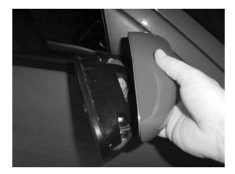
7. Next move to inside the door and using your fingers behind the small speaker panel, pop this cover off. To get access to the screws which hold on the mirror assembly.
