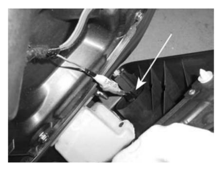
21. Now the inner door panel is free and cam be set aside until you are ready to put it back together. Note the courtesy light dangling in the bottom right corner of the picture. This is where you will tap into the circuit to power your puddle lamps.
