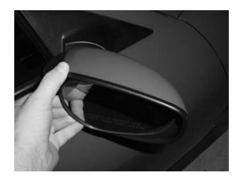
4. Three ball/socket connectors packed in grease hold on the mirror. You must continue pulling on the mirror to extract it from all three sockets. If you have heated mirrors you will need to disconnect the two leads (not shown).
