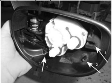
25. Insert the wire assembly through the slot as shown.
