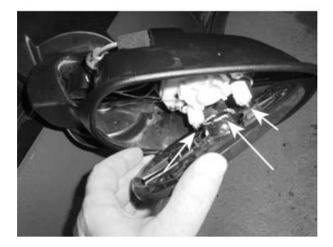
5. Once the mirror is removed from the sockets (easily seen here), the clips retaining the painted cover need to be released with a medium screwdriver to allow the cover to come off.
