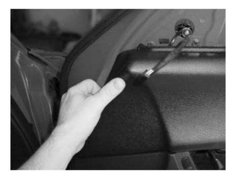
17. Once the nine clips are released, the door panel can be pulled off the door by lifting it straight up. The door panel "hangs" on the window opening so it needs to be lifted off the window opening to come free. CAUTION: There are still two wire assemblies that need to be disconnected before the door panel will be completely free. You just want to lift the door panel off the door.
