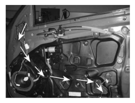
36. Using two of the wire taps provided, tap into the two wires running to the courtesy lamp as shown
