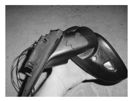
34. There is a retaining screw in the center of the mount panel. Loosen this screw and run the wires under the flat washer and re-tighten the screw. CAUTION: DO NOT OVERTIGHTEN THE SCREW AND CRUSH THE WIRES. Just make it snug to hold the wires in place.
