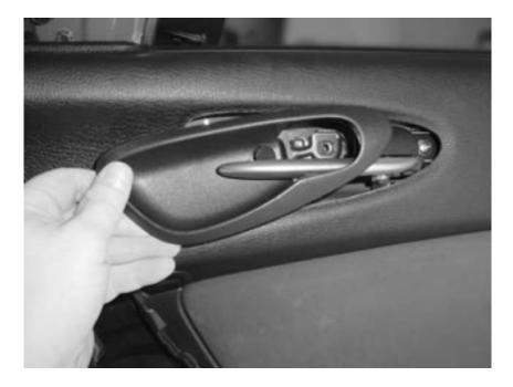
12. Next, you need to pry out the bottom of the window switch/door lock panel. Use a screwdriver covered with a small amount of masking tape to avoid scratching the piano black finish. Carefully pry the base away from the arm rest/handle panel.
