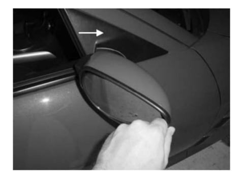
3. Push the outer edge of the mirror (the glass area) all the way in on the outside so you can get your fingers behind the mirror as shown. Pull on the mirror with steady pressure until it pops loose. You must be brave and don't be concerned about breaking it ... this is the way it is done.
