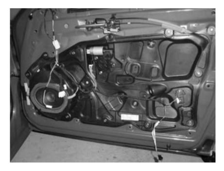
22. Disconnect the mirror wiring harness shown here located just below where you removed the speaker panel in step 6.
