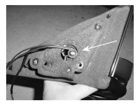
35. Replace the mirror on the doorframe using the three 8mm bolts previously removed. Plug the mirror wiring harness back into the socket from step 22. Run the puddle lamp wire assembly through the access hole and along the path shown to the courtesy lamp at the back of the door.
