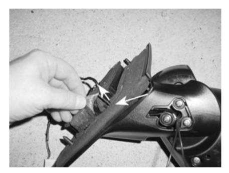
33. Once the wires have been run as indicated, the panel under the mirror assembly can be replaced
