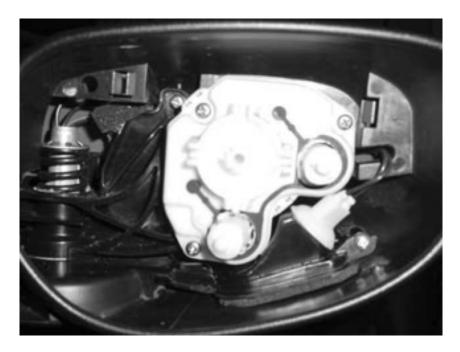
28. With the puddle lamp housing secured, turn your attention to the back of the mirror assembly. Route the wires under the clip as shown below.
