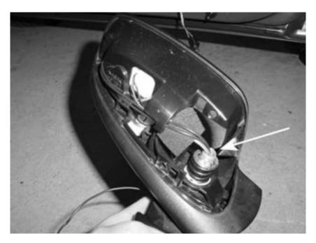
31. Following the path of the arrows shown, route the wires through the housing and under the foam insulation. You'll want to carefully peel back the foam insulation (as shown) to gain access to the hidden channel in the mirror mount plate.
