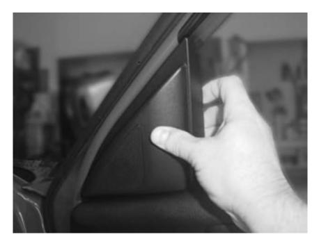
8. There is a wire and connector (see arrow) running to the speaker. You'll need to disconnect the connector to release the speaker housing and assembly
