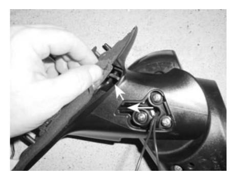
32. Continue routing the wires under the foam following the path of the arrows indicated. You'll need to peel back the second foam insulation pad to allow the wire to protrude through the center hole. You will see where the pre-existing wiring harness already travels this path, so just follow it with the puddle lamp wiring harness.
