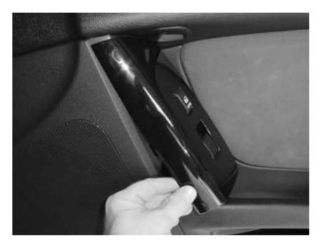
14. Once the panel is free, release the electrical connectors for the locks and window. The arrow indicates the location of the second screw that needs to be removed to get the door panel off.
