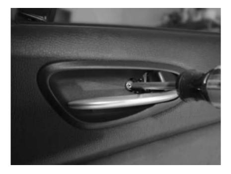
11. You can then remove the cover. You may need/want to pull on the handle just a bit to aid in removing this small cover. Note there are small plastic tabs used to hold the cover in place from behind, be gentle when removing the cover.
