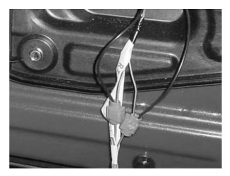
37. Using the wire ties provided, secure the puddle lamp wire harness to the existing wire harness at the points indicated by the arrows. Once they wires are secured you can cut the excess tab from each wire tie for a clean look.
