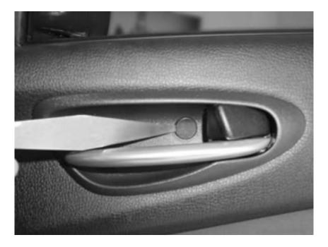
10. Then use a medium phillips screwdriver to remove the screw
