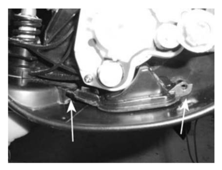
27. Before securing the puddle lamp housing, insert the bulb socket assembly into the housing and turn the plug 1/8<sup>Th</sup> of a turn to secure it in the housing. Note the orientation of the socket in the picture below. This is what it should look like to fit in the limited available space beneath the mirror motor assembly. Use the screw provided to secure the puddle lamp housing inside the mirror as shown.
