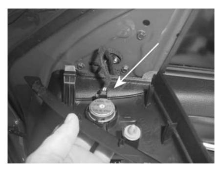
9. Next you'll want to remove the inner door panel, which is held on by 3 screws and several clips. In the door handle is a small round cover where the first screw can be found. Use a small screwdriver to pry the little round cover off.
