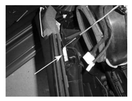
20. At the rear of the door is the courtesy lamp that needs to be pulled from the housing.
