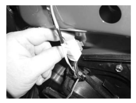
23. To remove the mirror assembly from the car you need to remove the three (3) 8mm screws located behind the speaker panel in Step 6. As you loosen the third screw, be sure to hold the mirror assembly so it does not accidentally fall to the floor. Carefully remove the mirror assembly from the door. CAUTION: There are plastic pins in the mirror housing used to locate the mirror assembly on the door. These pins can break if you are not careful removing the mirror assembly.
