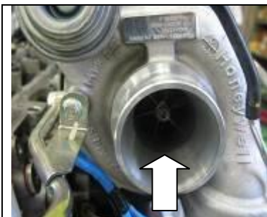
Visual inspection on the inside wall of housing
