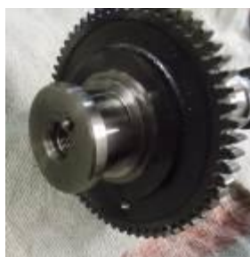
Camshaft locating pin pushed in
