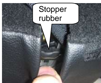
Rubber is correctly fit in position.
